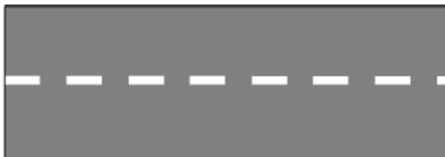
Figure 20 - Runway Centre-line Markings
