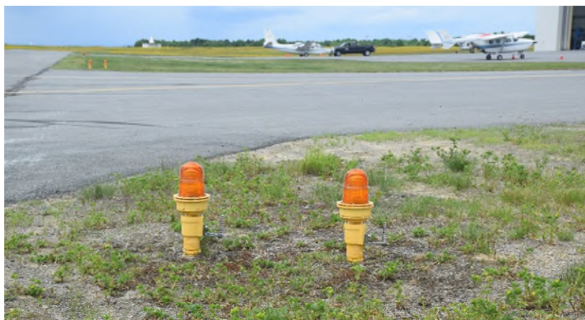
Figure 38 - Apron Entrance (Medium Intensity)
