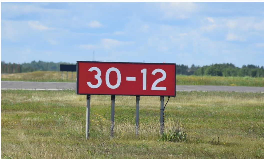
Figure 12 - Runway-Runway Intersection Mandatory Instruction Sign
